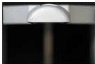
Figure 3a: View of optical finger probe on Index 2. The optical finger on the simulator does not accurately reflect the shape of a human finger.
